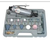
Die grinder features a powerful 1/2 HP motor, built-in power regulator, variable speed throttle control and full ball bearing construction. Standard with 1/4" collet. Specifications: 22,000 rpm; 1/4" collet; 5½" length; 14 oz. weight; 2 cfm average air consumption.
