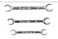
Ideal for gas, brake and air conditioning lines, flare wrenches provide more power and torque where needed. Tools manufactured with high-polished, heat-treated chrome vanadium. Three-piece set includes double-ended wrenches sized 10 mm x 12 mm, 13 mm x 14 mm and 15 mm x 17 mm. Available individually.
