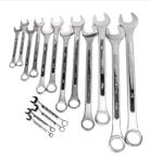
Made of drop forged steel, wrenches are chrome plated and heat treated to achieve maximum wear. A raised panel provides additional strength and durability. Sixteen-piece fractional set includes sizes 1/4", 5/16", 3/8", 7/16", 1/2", 9/16", 5/8", 11/16", 3/4", 13/16", 7/8", 15/16", 1", 1-1/16", 1-1/8" and 1-1/4". Packaged in kit bag organizer. Available individually.
