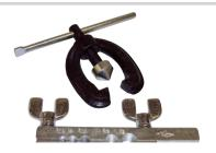
Professional double flare tool kit for fabricating double-compression lines (brake lines) or single-compression lines (fuel lines) in copper, steel, or aluminum. Kit features high-grade, alloy-steel center screw; plated, heat-treated, precision-ground swivel; and drop-forged, heat-treated yoke. Includes five adapters (3/16", 1/4", 5/16", 3/8" and 1/2"); each is laser engraved for easy identification. Packaged in blow-molded case. Adapters available individually. Weight: 2.3 lbs.
